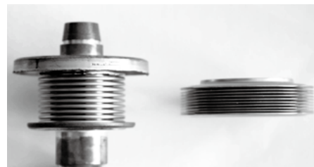
Comparison of steel sleeves: composed steel sleeve of TEL type, welded together from individual discs.
